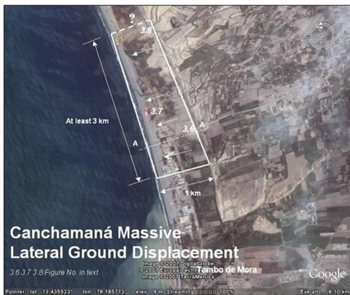
Figure 4. Approximate area of seaward lateral displacement of a marine terrace in Canchamana (background image from Google Earth).
