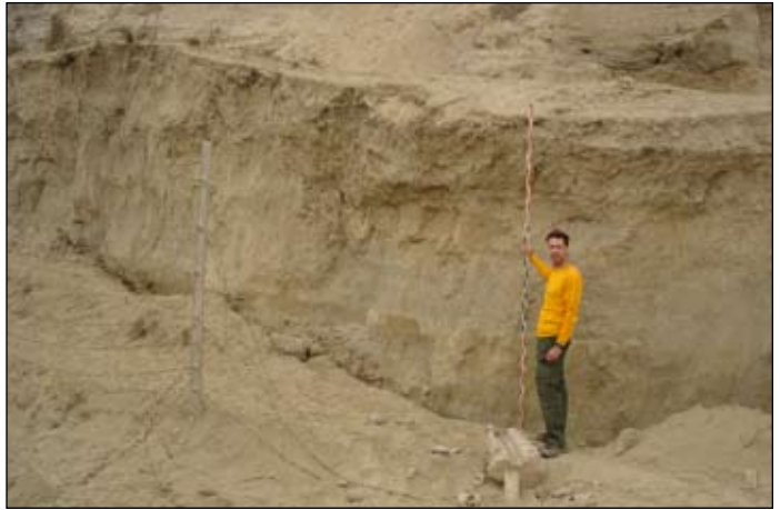
Figure 6. Maximum vertical offset of approximately 3.0 m along the interface between the marine terrace deposit and the Cañete formation in the Canchamana lateral slide.
