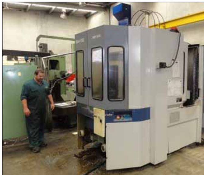
Figure 17. Equipment weighing 25,000 lbs moved approximately one meter (worker’s foot indicates the original position of the equipment) (photo: Marshall).
